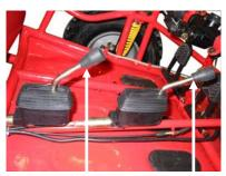
Gear Brake lever Lever
