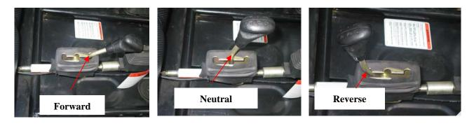
Never move the gear shift lever to reverse gear when the buggy is running, otherwise the engine and transmission will be damaged. Reduce speed before change to reverse gear.
