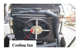
b. The engine cooling system is using closed cooling forced circulation system which mainly consists of radiator, sub water tank, water pump, heat-sensor switch, water holes, fan blade and fan motor.
