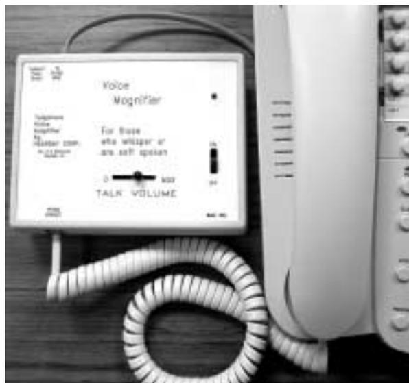
The **VM** is quick to attach to a phone and is small enough to take along with you to use with a phone at work, at a friend's or relative's home or in a hotel room. Measures 5.7" x 3.6" x 1.5" Weighs 8 oz. with a 9 V. alkaline battery inserted.
